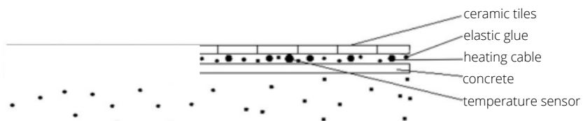
Figure 2: Directly on the concrete
